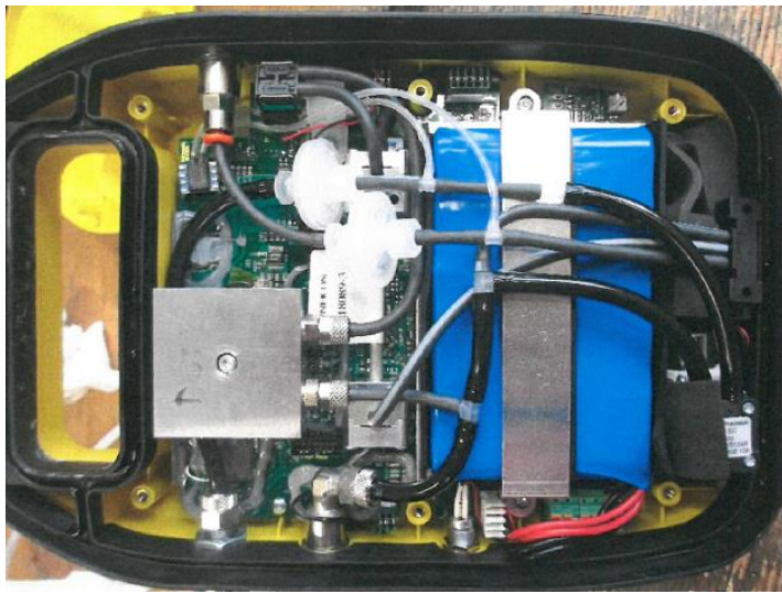
View inside after IP 54 test.
